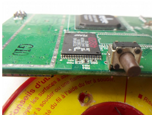
Picture 14: slightly misaligned chip with a bent lead, still acceptable though (WRE54G V1.0)
