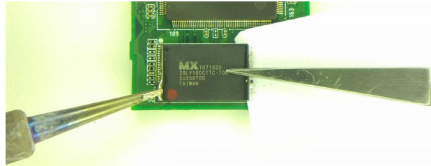
Picture 6: desoldering the other side, the chip is held with tweezers
