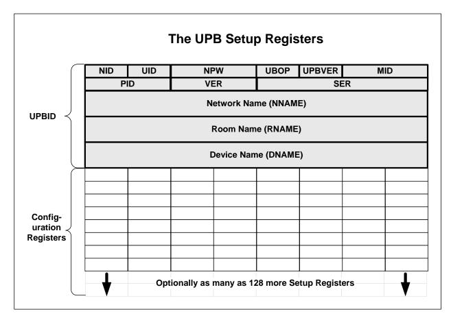
Figure 10: The UPB Setup Registers
