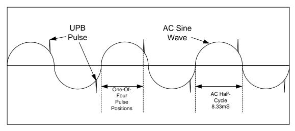
Figure 1: UPB Pulse Communication Method
