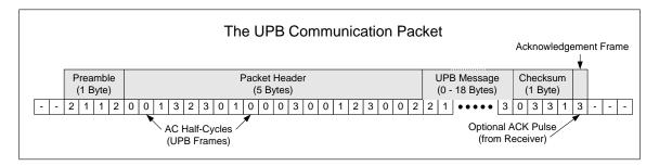
Figure 4: The Standard UPB Communication Packet
