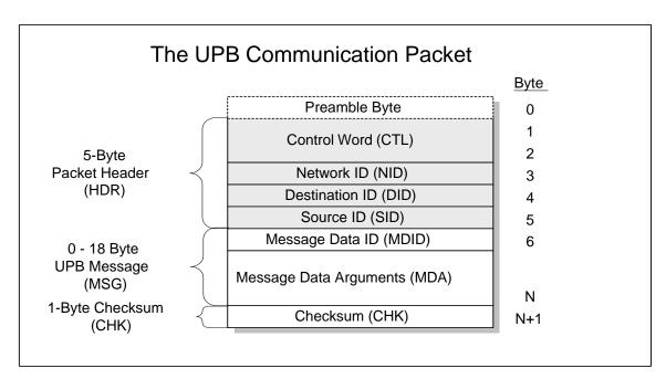
Figure 5: The Packet Header
