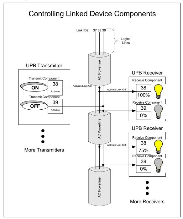
Figure 13: UPB Device Component Linking Example
