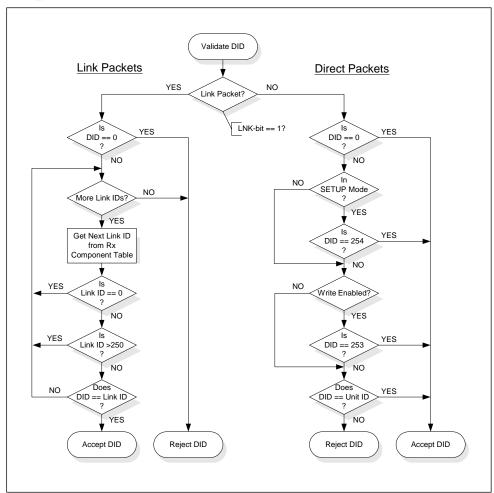
Figure 6: Destination ID Validation Process
