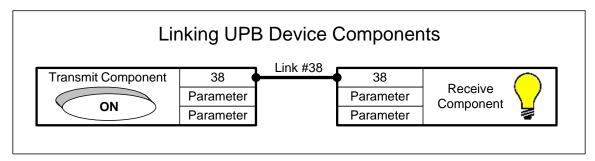
Figure 12: Linking UPB Device Components
